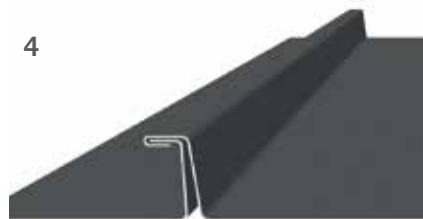
First turn completes angle standing seam joint
