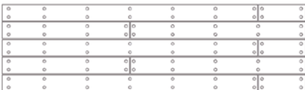
Open gap boarding laid in a staggered configuration
