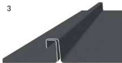
Small gap at base forms automatically and allows for lateral thermal expansion
