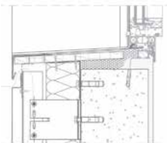
Vented window sill
