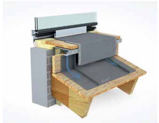
DLSS 6.1.01 – Vented abutment (under window).
