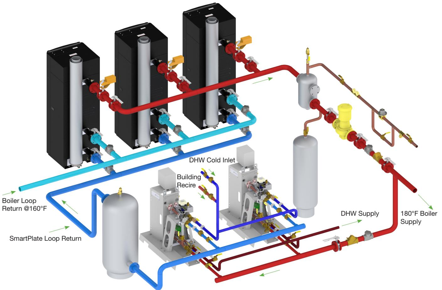
Additionally, for a dual inlet boiler like AERCO's Benchmark series, the efficiency gain would be even higher (3% to 5.5% on average) as shown in the charts below at full fire and minimum fire rate.
