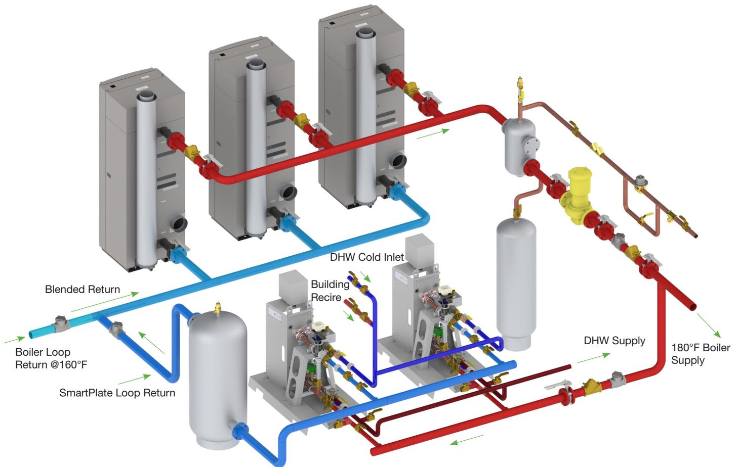
Combination Plant: SmartPlate for DHW solution increases boiler efficiency.
