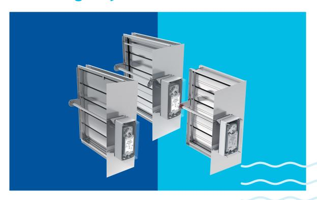
Genset dampers are designed to provide maximum combustion air and pressure relief quickly for emergency generator start up to avoid damage of equipment or surrounding space. Ruskin offers three genset options including the CD50GS, CD60GS, and TED50GS. All of which have Class 1A Leakage performance to save energy and special fast acting 8 second spring-return actuators tested to 40,000 cycles.
