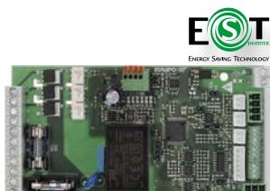
OPower-card for brushless motors for BMS (built-in the unit)
