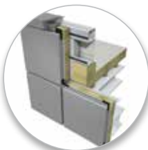
TOP PARAPET DETAIL
