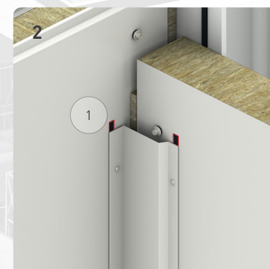
Fig. 4.7: TE-H-05.01 internal corner sealing elements
