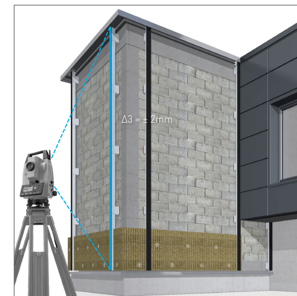
The measurement procedure for ensuring the vertical alignment of the substructure for horizontal installation.
