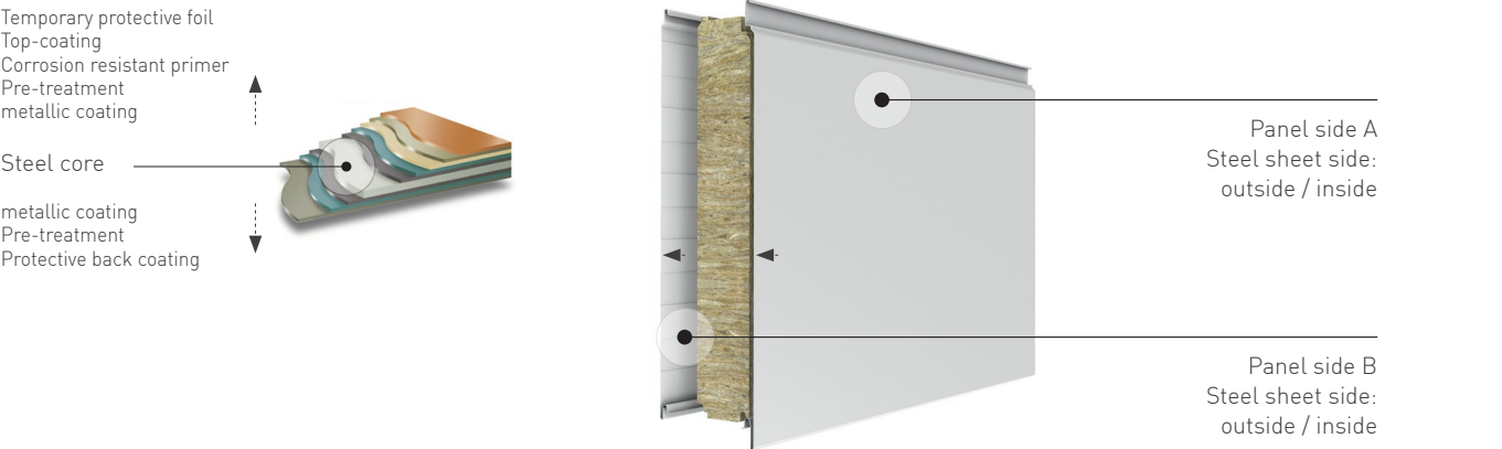
Fig. 2.1: Panel composition and coating structure example
