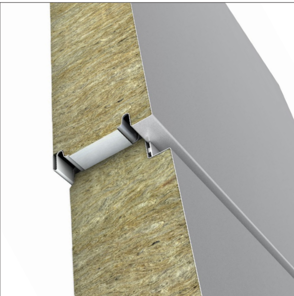
Correct sealing in both longitudinal joints
