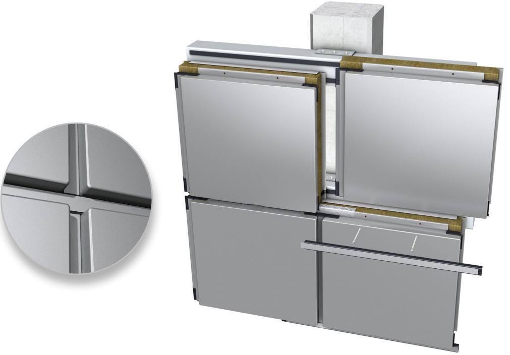
Qbiss One B-B vertical element joint detail
