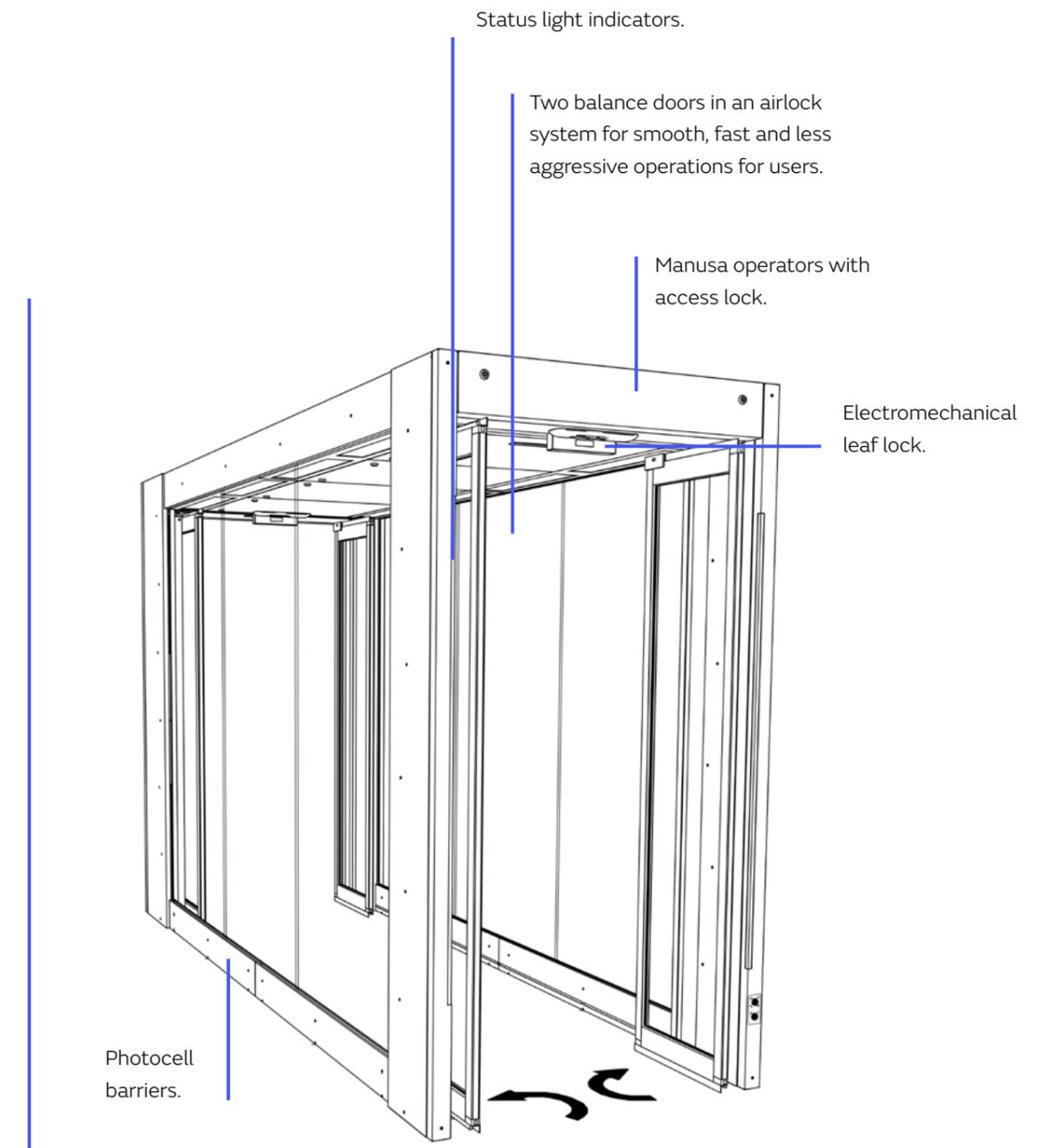
With in-house technology, the one-way corridors can be configured and scaled in individual or multiple mode in parallel, and the assembly is entirely self-supporting and easy to maintain.
