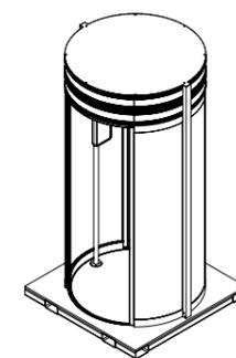
**Airlock system with circular sliding door**
