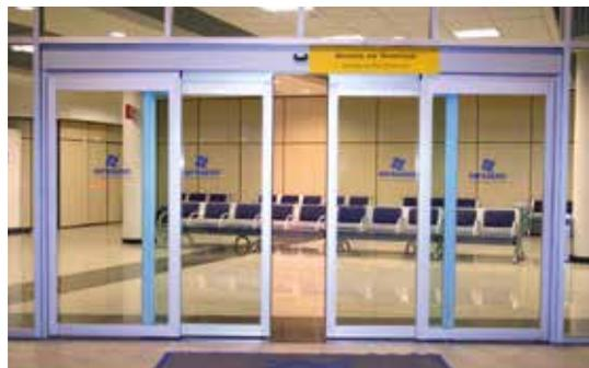
**Panic break-out system with framed leaves (A45-S4):** sliding and break-out leaves with them fully framed with a 45 mm frame offer high resistance and durability, which makes it suitable for high traffic sites.
