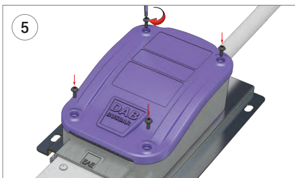
5- Refit the Feed Box cover by replacing the screws as shown. Be sure to use "U" support for the installation.
