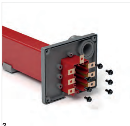
2 Screw the conductors to the feeding module. Connect the feeding cables by putting them through the cable gland.
