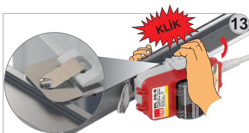
First, connect product earth terminal to busbar plug-in point. Then make sure that other terminals connect to busbar. Finally you should hear "CLICK" sound when you press tap-off box towards busbar.
