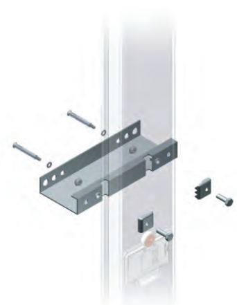
Vertical Shaft Installation
