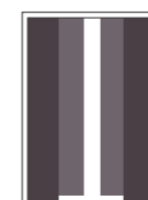
Porta scorrevole interno muro ante sovrapposte doppie Inside the wall sliding door with two overlapping double leaves
