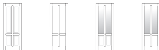
cieca con bugna blank with raised panel cieca con foderina blank with flat panel finestrata con bugna glazed with raised panel finestrata con foderina glazed with flat panel
