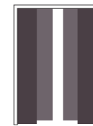
Porta scorrevole interno muro a 2 ante sovrapposte doppie Inside the wall sliding door with two overlapping double leaves
