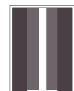
Scorrevole interno muro 2 ante sovrapposte doppie Inside the wall sliding door with two overlapping dou- ble leaves
