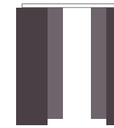
Scorrevole esterno muro 2 ante sovrapposte doppie Outside the wall sliding door with two overlapping double leaves
