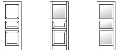
cieca con pannello blank with panel finestrata con bugna glazed with raised panel finestrata glazed
