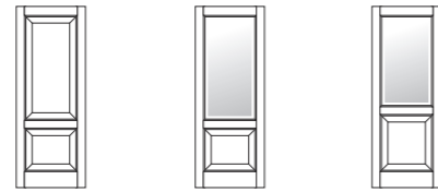
cieca con bugna blank with raised panel finestrata con bugna glazed with raised panel finestrata con bugna glazed with raised panel
