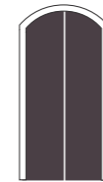
Porta a due ante ad arco a sesto ribassato Double leaf with lowered arch
