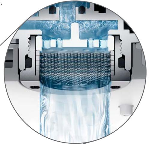
Utilizing a unique interior structure, the flow of water is controlled to provide a smoother shower.
