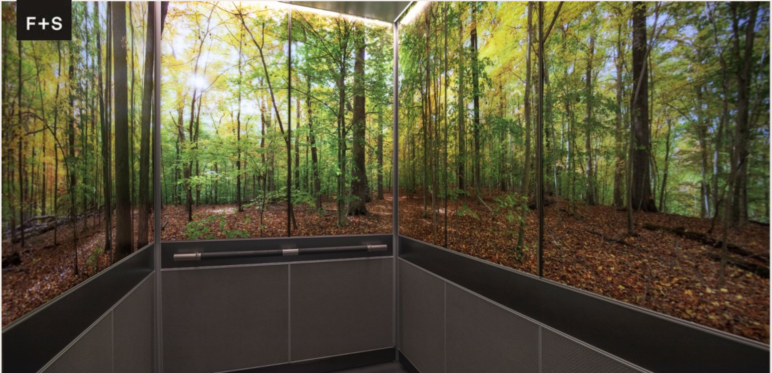
LEVELe Elevator Interior, LightPlane Panels, ViviSpectra Zoom glass, Bonded Metal, Fused Nickel Silver. Sextant Handrail | 11645 Wilshire Blvd
