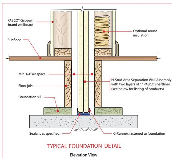
**Note:** C-runner must be positioned a minimum of 3/4-inch from adjacent framed interior wall that will support the aluminum breakaway clips.
