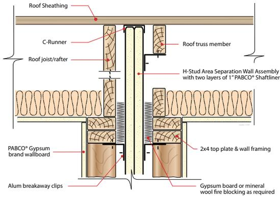
**TYPICAL ROOF INTERSECTION DETAIL**
