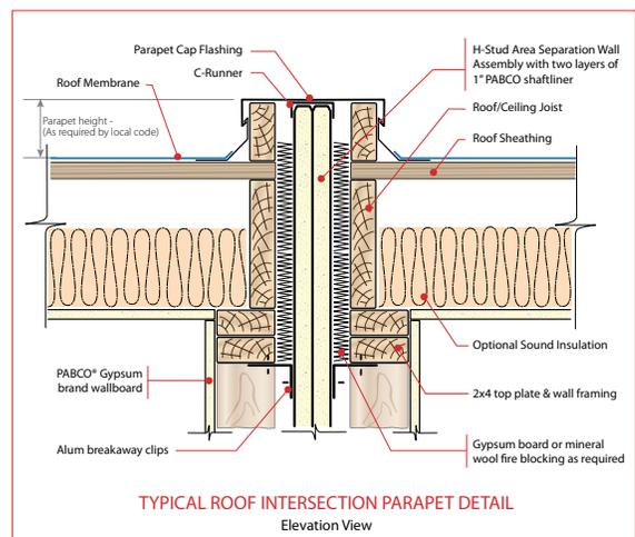
**Note:** When the total height of the ASW exceeds 44 feet but not more than 66-feet, the vertical spacing between the rows of the L-Shaped aluminum breakaway clips shall not exceed 39 inches. When the total height of the ASW is less than 44 feet, the vertical spacing between the rows of the L-Shaped aluminum breakaway clips shall not exceed 60-inches.
