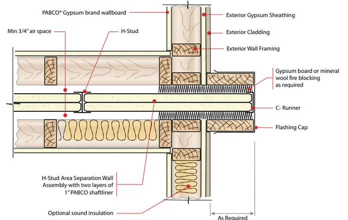
**PROTRUDING EXTERIOR WALL INTERSECTION DETAIL**
