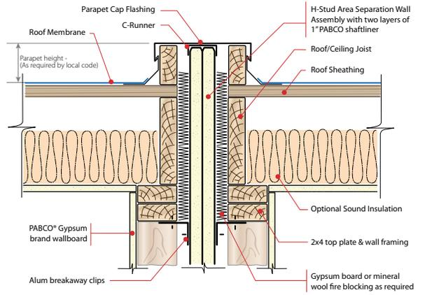
**TYPICAL ROOF INTERSECTION PARAPET DETAIL**
