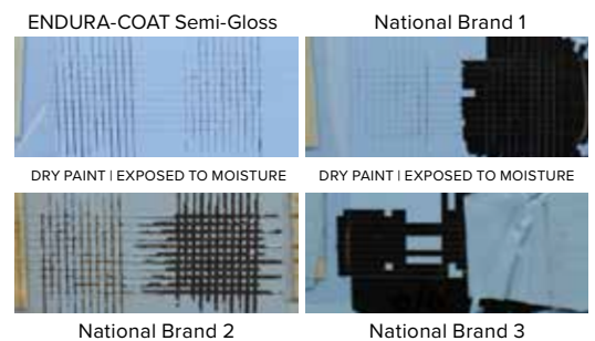
Adhesion refers to the ability to bond firmly to the substrate and create a stable foundation for topcoats.
