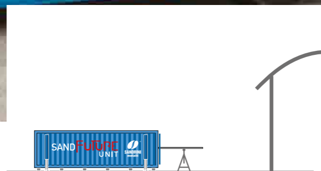
PROFILATURA CON SAND FUTURE UNIT A TERRA GROUND-BASED ROLL-FORMING WITH THE SANDFUTURE UNIT
