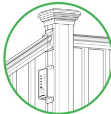
Do not install Control Hub in direct view/close proximity of post cap lighting, as it will cause undesired results.
