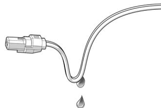
It is our recommendation that a "drip loop" be created during wire routing. Above is an image of how to properly orient the wires.
