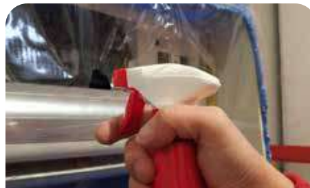
Battery cleaning through spraygun hole
