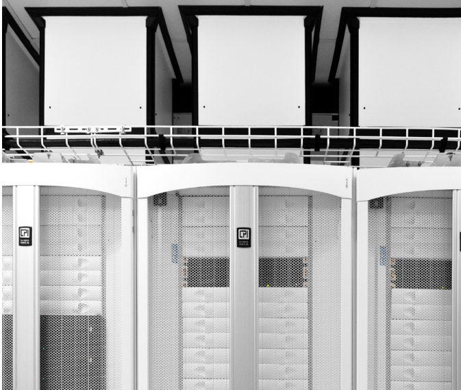
CPI's Vertical Exhaust Ducts guide hot exhaust air from the back of the cabinet to the drop ceiling plenum, creating a closed hot air return path to the cooling system.
