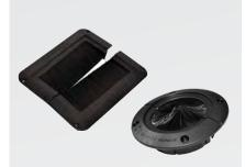
Figure 5: Raised Floor Grommets are available in various sizes and shapes. They seal openings in raised floor tiles with brushes or rubberized gaskets to reduce air leaks around cables, conduit and piping. Use these grommets to seal openings in raised floor tiles when the interstitial space under the floor is used as a supply air plenum.
