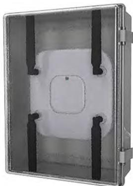
The easy-to-install model 1024 NEMA 4 enclosure features a hinged, lockable lid. A universal interior mount panel will accommodate all leading vendors' APs. This rugged, polycarbonate, low-loss enclosure is available with either a clear or opaque door and is large enough for AP with attached antennas. Ideal for Wi-Fi coverage in parking areas and garages.
