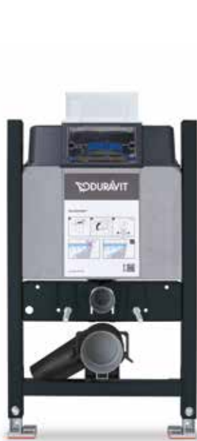
Toilet frame Standard Basic 84cm # WD1017 000 000 In-wall cistern, maximum flushing volume 9.0 l, insulated against condensation, incl. SensoWash®-prepared. Operated from the front or from above. Suitable for dry-wall installation
