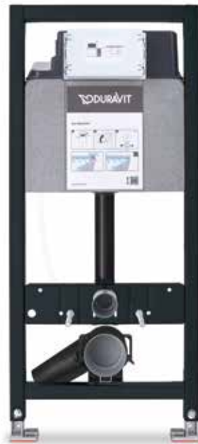
Toilet frame Standard Basic 115cm # WD1020 000 000 In-wall cistern, maximum flushing volume 9.0 l, insulated against condensation, incl. SensoWash®-prepared. Operated from the front. Suitable for dry-wall installation
