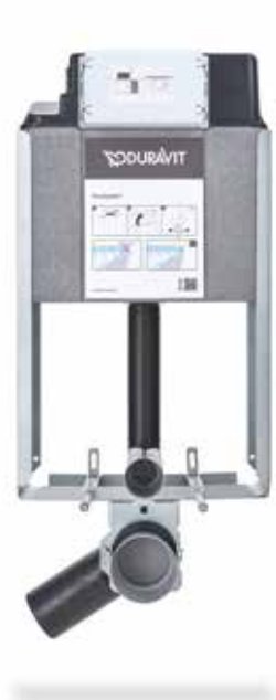
Toilet frame Standard Basic for wet installation # WD1015 000 000 In-wall cistern, maximum flushing volume 9.0 l, insulated against condensation, incl. SensoWash®-prepared. Operated from the front. Suitable for dry-wall installation.
