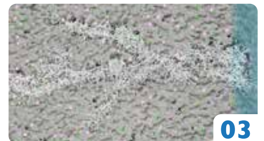
Crystals seal and block capillary pores, preventing any further water ingress.
