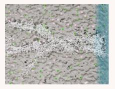
These crystals seal concrete pores and capillary cracks up to 0.4 mm wide, preventing water and various chemicals from entering the concrete mass.
