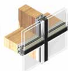
4-Sided Structurally Glazed Wood Facade
