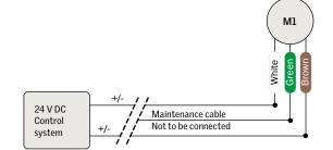
Connection to a fieldbus system requires a separate control box between fieldbus system and actuator. For the OS  $\pm$  24 V DC, only the actuators are supplied by the VELUX Group.
