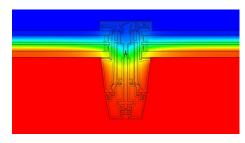
Thermal tests reveal the profile's ability to prevent cold bridging.
