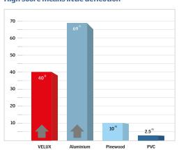
The high rigidity of the pultruded composite material makes the frame and sash extremely stiff. The rigid properties ensure reliable performance with very little deflection of the profiles and more durable aesthetics.
