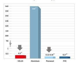
The special composite possesses extremely low-conductive properties that surpass traditional profile materials - a measure for high insulating performance.
