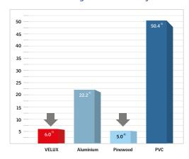
Traditional skylight materials fluctuate in form due to thermal changes, causing damage to gaskets and an increased risk of water ingress. Since the modular skylight composite contains 80% fibreglass, the profile properties are quite equal to those of the glazing unit. The similarity minimizes the risk of opposing movements in the construction, ensuring tightness of joints and a longer life expectancy of the application.
