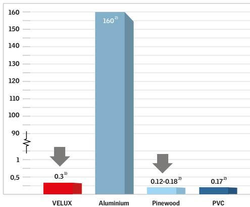
The special composite possesses extremely low-conductive properties that surpass traditional profile materials – a measure for high insulating performance.
