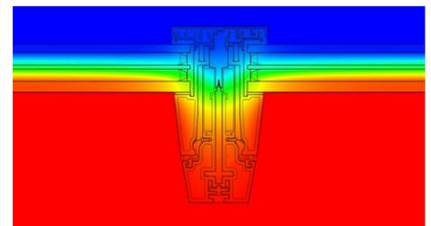
Thermal tests reveal the profile's ability to prevent cold bridging.
