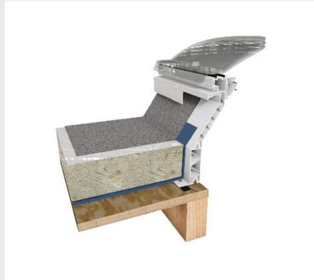
Dome Rooflights can be fixed directly to the roof, or they can be used with an upstand for maximum weatherproofing. They are suitable for use with all standard roofing membrane systems on roofs with pitches of up to 15°.
