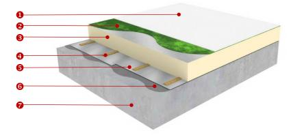
Elevate's TPO Fully Adhered System is a lightweight system with outstanding design flexibility. It is suitable for contoured roofs, roofs with irregular shape and any roof with limited load bearing capacity, provided the substrate is compatible with Elevate contact adhesives and provides sufficient adhesion.
