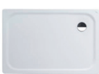
PLATINA H215005...xxx1 Shower tray, rectangular, enamelled steel (3.5 mm), extra flat (30 mm)
