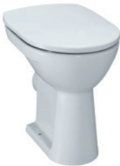
H825956...xxx1 Floorstanding WC 'comfort', washout, with flushing rim, outlet horizontal, sitting height 450 mm
