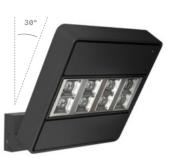
Available in three finishes: white, silver-grey and dark grey. Suitable for installations up to 40 metres in height. It comes in an IP66 IK10 version designed for outdoor and highly exposed spaces. It offers three different optics—emergency escape routes, open area and wall—with proprietary lenses that fit into an aluminium reflector.
