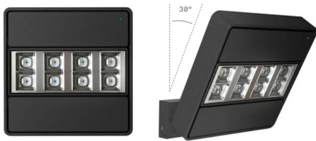
Available in three finishes: white, silver-grey and dark grey. Suitable for installations up to 40 metres in height. It comes in an IP66 IK10 version designed for outdoor and highly exposed spaces. It offers three different optics—emergency escape routes, open area and wall—with proprietary lenses that fit into an aluminium reflector.
