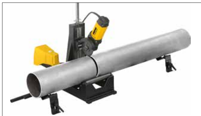
Figure 12 - Cutting the pipe to length
