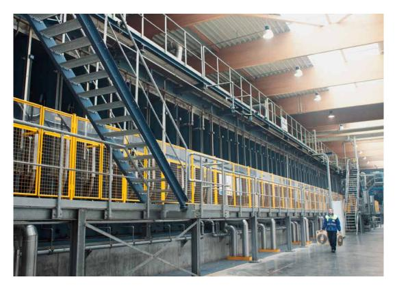
The ContiRoll press: The centrepiece of every EGGER plant for the production of rawboard. The installation shown here in Hexham (UK) is 48.5 m long and 2.6m wide. It is in operation around the clock.
