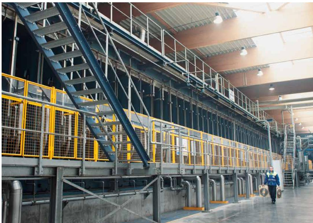
The ContiRoll press: The centrepiece of every EGGER plant for the production of rawboard. The installation shown here in Hexham (UK) is 48.5m long and 2.6m wide. It is in operation around the clock.
