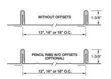
\*24 gauge steel, in all O.C.'s is UL-90 Classified over solid substrate. See roof deck construction in Underwriter Laboratories roofing materials and systems directory.
