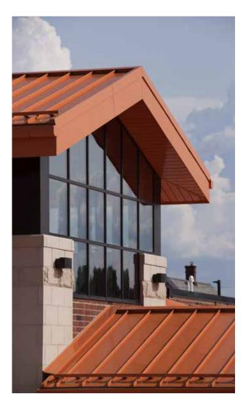
Redi-Roof standing seam is intended for application over a solid substrate with a minimum 3:12 roof pitch. Typical substrates include plywood, nailboard insulation or equal. Panels are factory roll-formed in continuous lengths. Maximum panel length is 45' and minimum panel length is 4'.
