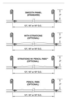
Not all panel conditions are available in each Petersen branch; additional freight charges might apply if specific panel condition is required. Tite-Loc and Tite-Loc Plus panels are supplied "smooth" as standard. Customer must advise if additional panel conditions are required.
