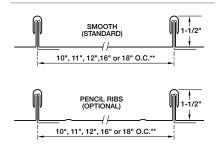
\*12" and 18" 24 gauge steel Snap-On Standing Seam panels and 11" and 18" 24 gauge steel High Snap-On Standing Seam panels are UL-90 Classified over solid substrate. See roof deck construction in Underwriter Laboratories roofing materials and systems directory.
