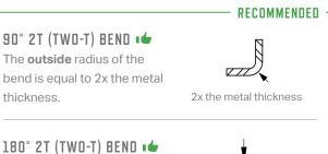
The **inside** radius of the bend is equal to 2x the metal thickness.
