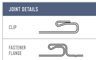
Box Rib panels should be installed in single-piece runs, either horizontally or vertically. For panels more than 20-ft. long, the clip version should be utilized. For panels less than 20-ft. long, the screw leg version is acceptable. For wall elevations with panels longer than 36-ft., flashing breaks must be used as indicated by the architect or designer. Box Rib panels are NOT designed to be field-lapped over one another.
