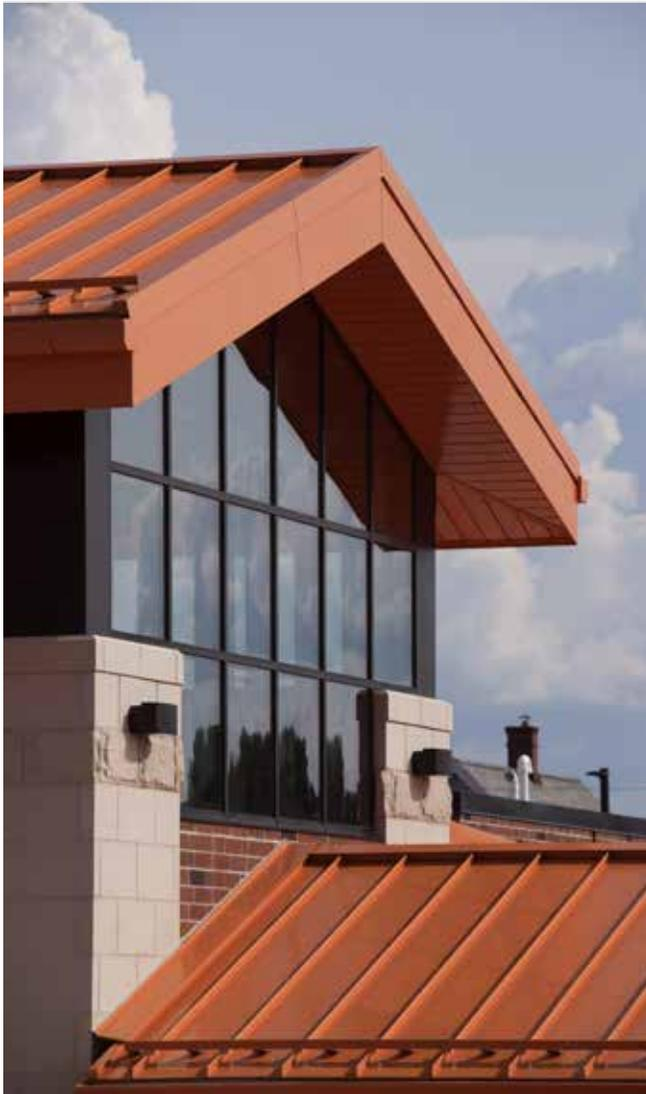
Redi-Roof standing seam is intended for application over a solid substrate with a minimum 3:12 roof pitch. Typical substrates include plywood, nailboard insulation or equal. Panels are factory roll-formed in continuous lengths. Maximum panel length is 45' and minimum panel length is 4'.
