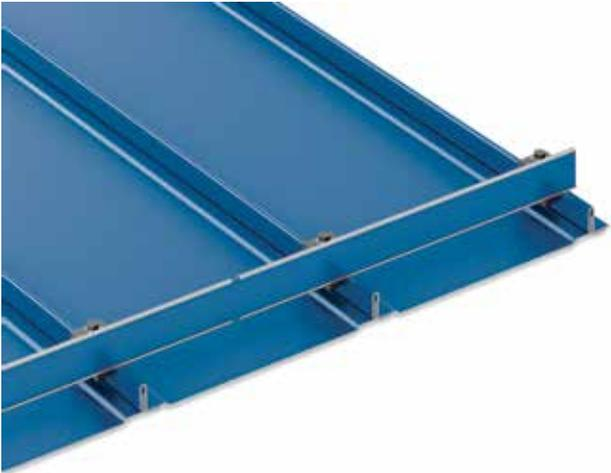
Petersen is stocking the patented ColorGard snow retention system. ColorGard is the only product available which will precisely match the color of any Petersen roof panel. ColorGard achieves this by utilizing a strip of the roof material, which is then mounted directly into ColorGard for a perfect match. This strip can be cut in the field or at Petersen's factory.
