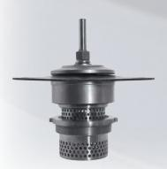
Ames optional Polyjet Trim greatly reduces the damaging effects of cavitation by utilizing multi-staged energy dissipating technology. Its proven design is ideally suited for extreme differential pressure situations including Pressure Reducing, Pressure Relief and Reservoir Fill Applications.
