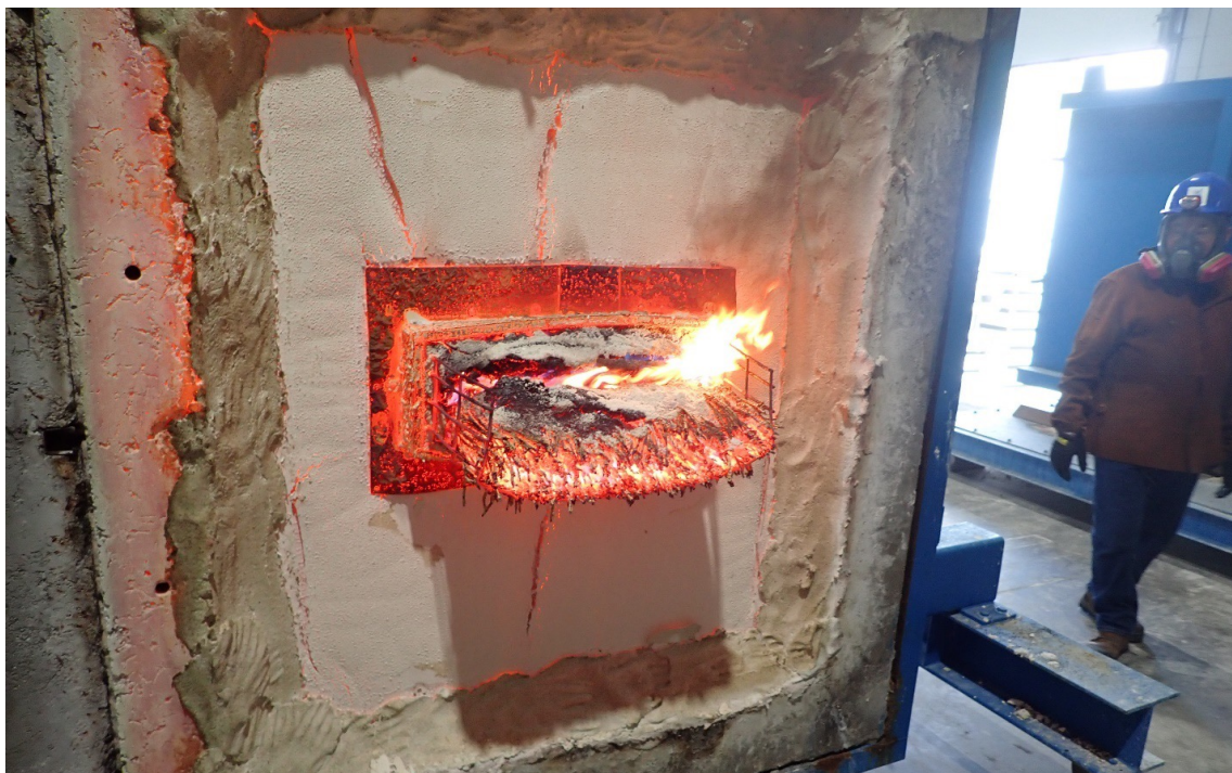
EZ Path® Cable Tray Retrofit Device Upon Completion of Fire Endurance Testing (W-L-4102)
