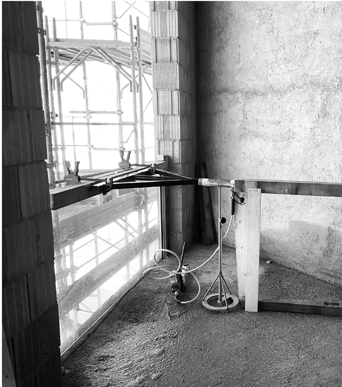
Example of an on-site test with static load test up to 300 kg/m (202 lb/ft) with a 10+10 (3/8"+3/8") glass 250 cm (98.4") wide and 110 cm (43.3") high, with totally positive results.
