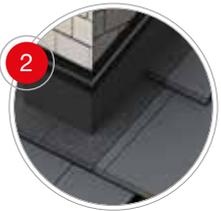
To adequately solve roof joints and chimneys, multi-use (Premium or Aluminium) waterproofing bands should be used. Once attached to the clean dry surface, they must then be finished with the Counter flashing profile, sealing the upper line with a continuous line of putty.
