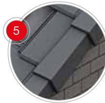
Edges clay accessory (left and right) should be installed overlapping the roof tiles and following the direction of the tile. To complete the slope on the left it should be placed on the roof tile or half-tile, depending on the width of the roof surface and method of installation (straight or in staggered formation).
